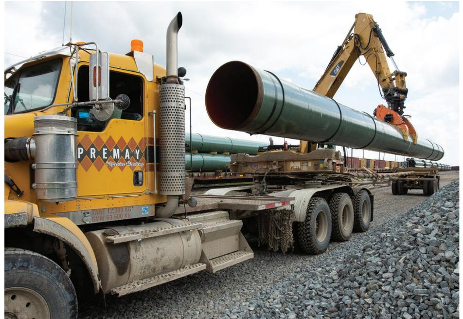
jobsites during the summer of 2006. Originally designed in 1999, vacuum lifts were designed to use a diesel motor powering a suction pump to create a seal between the attachment and the pipe, thereby allowing an operator to move pipe using an excavator.
